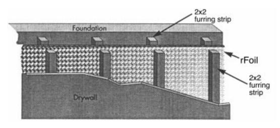
(It is important to remember that rFoil works best when there is a 1" airspace between rFoil and another material, like drywall or paneling. Since it is important to block heat leaving a building or house, the 1" airspace should be closest to the inside).
